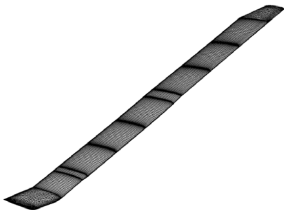
Figure 26. UH-60A rotor blade surface mesh.
