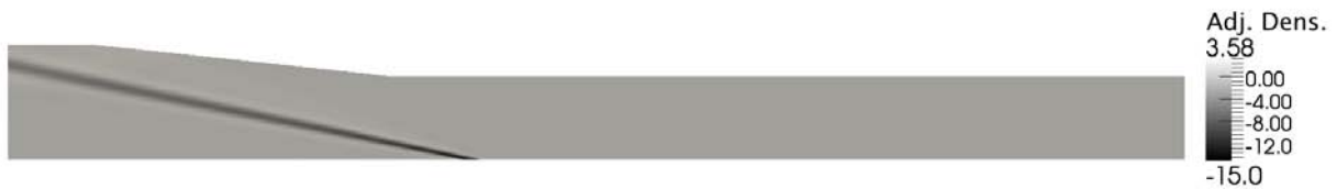
Figure 61. Density contours for nominal conditions (inflow Mach number 5.0 and ramp angle 6.0°).
