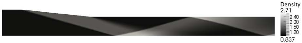
Figure 61. Density contours for nominal conditions (inflow Mach number 5.0 and ramp angle 6.0°).
