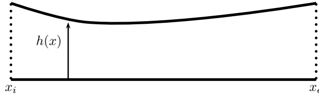
Figure 4. Quasi one-dimensional duct
